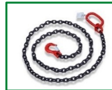
Article-no.: 211308 Choker Chain 8 mm, 3 m long max. capacity 4 t Breaking load 8 t
